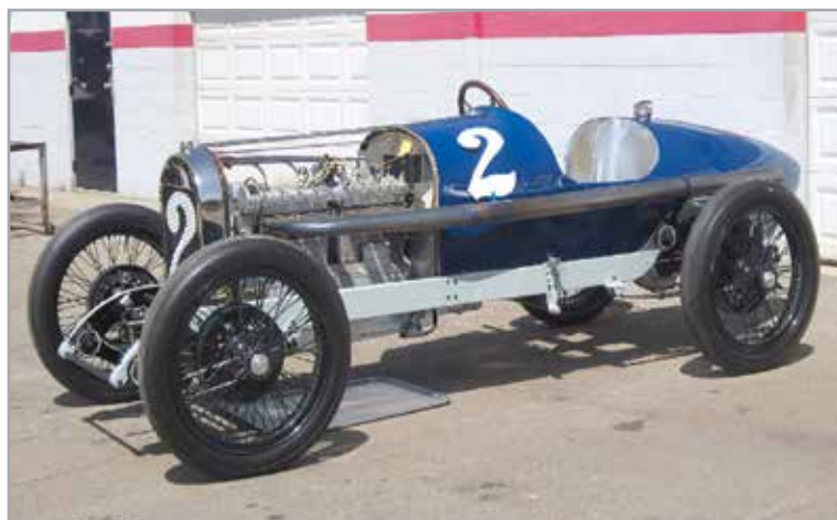
Brent Castle's Milton-Durant Special, the first Miller 4-cylinder chassis, with 8-cylinder 183 engine #2 or #3.
