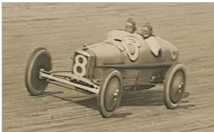
Tommy Milton in 1922 with the third 8-cylinder 183 engine in his Miller-built cross-spring chassis.
