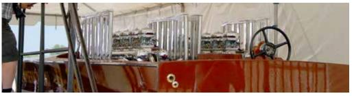
The 1929 Gar Wood Miss America VIII Boat – Two-time winner of the British International Harmsworth Trophy, the top prize for unlimited power boats. Features 1931 specially designed Harry Miller V-16 1,113/930 HP (without original superchargers currently installed) one-off engines, with 6,000 RPM double overhead cam, aluminum block and heads. This extraordinary boat is owned by Dana Mecum.
